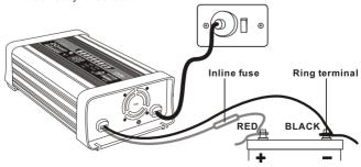
If the charger is used in a Permanent / Hard Wired application and the vehicle will not be used for sometime, it is best to leave the charger connected to mains power (turned "On") so that it can maintain the battery fully charged.
